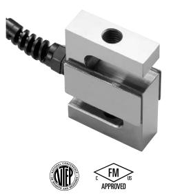
The S-type load cell, as the name indicates, can be easily identified by its S-shaped body. They can be loaded either in tension or compression, and used for single or multiple-cell application if the output is rationalized.
