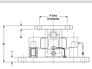
This mount is designed for a uniformly distributed load on the top and bottom surfaces
