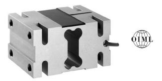
A special humidity resistant protective coating assures long-term reliability. The two additional sense wires feed back the voltage reaching the load cell. Complete compensation of changes in lead resistance, due to temperature change and/or cable extension, is achieved by feeding this voltage into the appropriate electronics.
