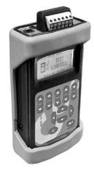
**Measurement Function:** Show mV output, excitation voltage, mA outputs for systems, etc.
