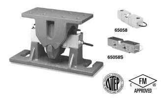
This product is designed to simplify the installation of the 65058 load cell into a certified Legal-for-Trade high capacity weigh bridge. Unilink<sup>™</sup> floating suspension allows controlled floating of the scale deck, providing a reliable and accurate weighing system. The load cell is nickel plated or stainless steel and sealed to IP67 standards, assuring reliability. The mount assembly is provided with a primer coat finish to simplify the manufacture of the scale.
