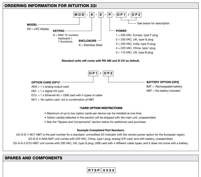
RTSP0070 = Bracket for option cards (supports up to two card slots) RTSP0580 = USB and Ethernet card installation kit RTSP0590 = Analog output card installation kit RTSP0600 = Digital I/O card installation kit RTSP0090 = Rechargeable battery RTSP0870 = RS485 card installation kit
