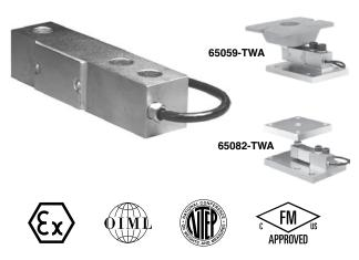
It has high immunity to shock or side loading and is available in 2 or 3 mV/V sensitivity. Approved to OIML and NTEP standards. For hazardous environments this load cell is available with EEx ia IIC T6 level of European approval.
