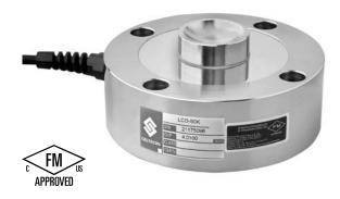
The low profile compression disk is designed as the ultimate solution for some difficult applications in which height is a major safety concern. The shear web design provides excellent performance even when side force inevitably exists in normal operations. A typical example of such side force can be found in motor truck scales, making the model LCD perfect for such applications.
