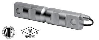
This product is designed for use in industrial and outdoor environments. Nickel plated steel construction limits corrosion from outdoor use. The IP67 sealing makes it suitable for applications that are subject to high-pressure wash down. Tank weighing is made simple when this load cell is combined with the EZ mount mounting hardware it was designed for. Its high accuracy and availability in high capacities make it ideal for certified truck and rail scales.
