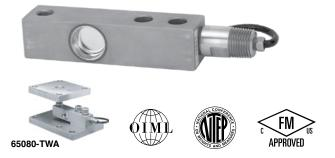
Its low profile and fully welded sealing combined with high accuracy makes this load cell ideally suited for low profile platforms, pallet truck weighers, tanks and silos. The guide slots incorporated into the upper and lower mounting faces enable manufacturers to easily position the load cell.
