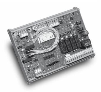
the limit set. It boasts a redundant safeguarding system that allows the load cells to be connected as independent pairs. The WG3 also features an integrated alarm for detecting load cell malfunctions or power failure, and a 60°C operating temperature range
